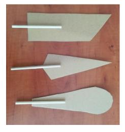
Blades typically consist of a wooden stick and a piece of cardboard. It would be best to glue the stick to the cardboard, but it can also be attached with an insulation tape. It's most important to attach it strongly so that the blade doesn't break apart when rotating at high speed.
