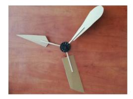
Rotor is assembled by putting the blades in the right holes of a hub. Design of a rotor depends on a number of blades used. There are 12 holes in the hub, so you can use 2, 3, 4, 6 or 12 blades to construct a symmetric and balanced rotor. Make sure you use the right pitch angle.
