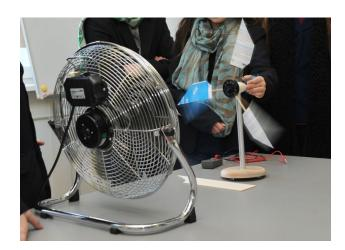
Wind turbine model test equipment consists of a fan and a multimeter. Also you can use a portable anemometer to assess wind turbine output under different wind speeds.
